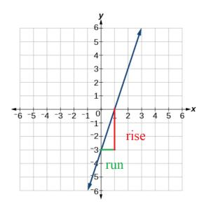
The slope is the ratio of rise to run.
